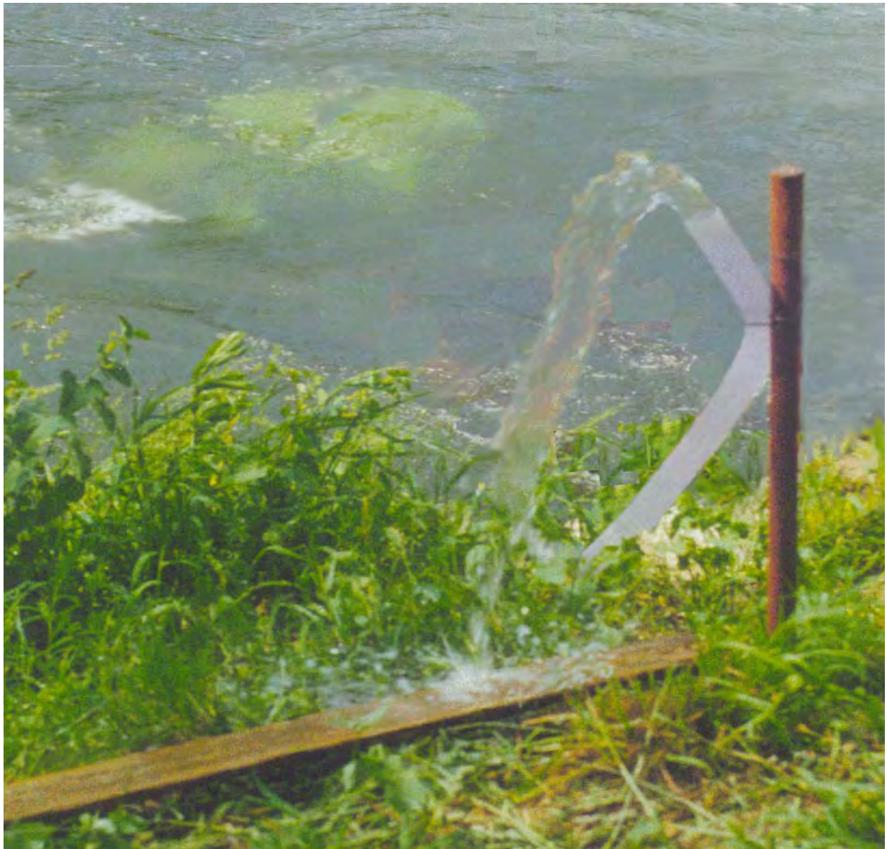
Several years ago, (due to centrifugal pump) the second prototype was able to deliver only 1 liter/second of water based on 1,2 bar of pressure.
